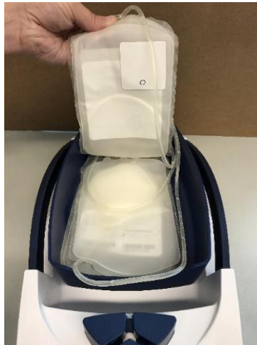
Figure 26: RFID tag position on middle bag
