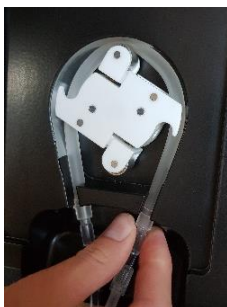
Figure 10: Insert pump segment
