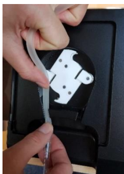
Figur 8: Sette inn pumpesegment
