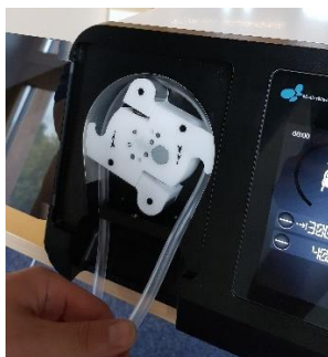
Figur 20: Slangesett i holder
