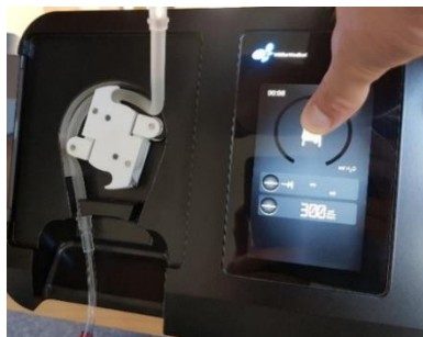
Figur 9: Vikle inn pumpesegmentet
